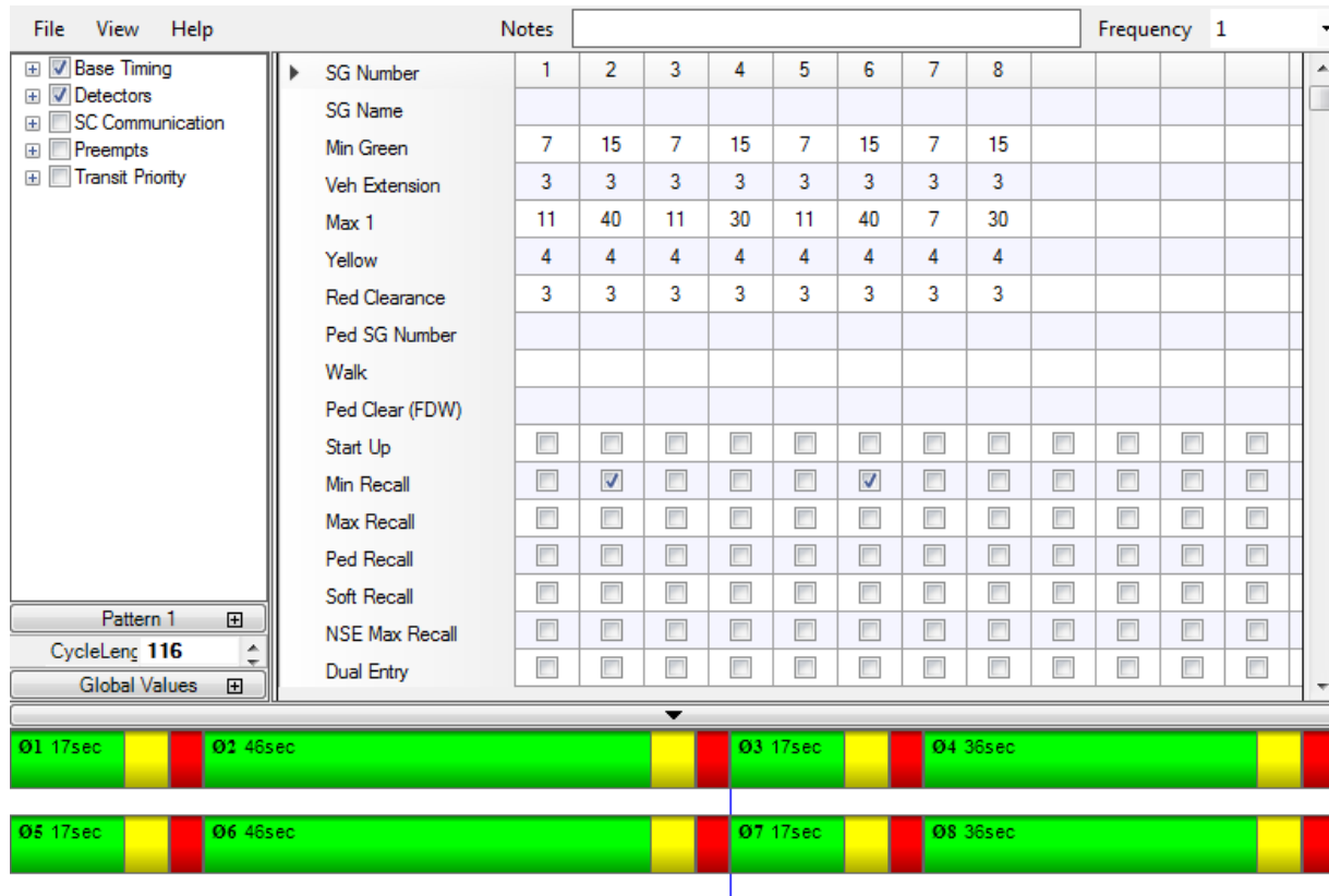
Figure 6: Actuated Controller Timing
